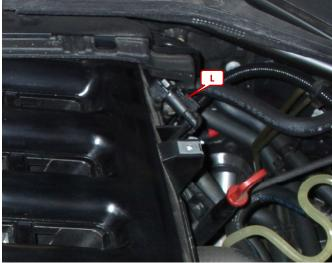
To disconnect the 3 pole boost pressure plug (L) press the locking lever. Connect the boost pressure adapter (L) between the both connections.
