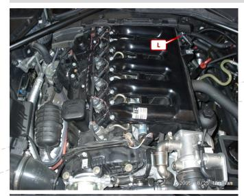
Localise the boost pressure sensor (L). The boost pressure sensor (L) is located top right next to the engine.
