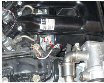
To disconnect the rail pressure plug press the locking lever. Connect the rail pressure adapter (R) between the both connections.
