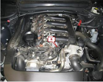
Localise the 3 pole rail pressure sensor (R) which is located in front of the common rail bar.
