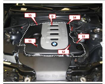
Open the engine hood. Solve the 5 hexagon socket screws (S1 – S5). Remove the engine cover (D).
