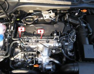
Localise the 3 pole rail pressure plug (R). It is located on the left side of the common rail bar (B).
