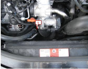
The boost pressure sensor (L) is located in front of the engine at the suction pipe.
