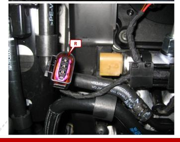
To disconnect the rail pressure plug (R) press the locking lever. Connect the rail pressure adapter between the both connections.
