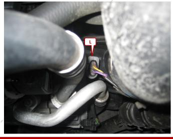
To disconnect the 3 pole boost pressure plug (L) press the locking lever. Connect the boost pressure adapter between the both connections. Connect the CRD module with the adapter cable. Check all connections again and reassemble the vehicle in reverse order.
