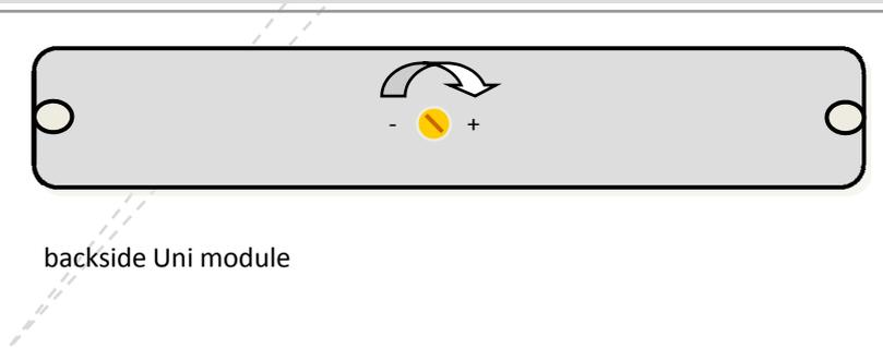
To increase the curve turn the potentiometer clockwise. Drive extensively test.
