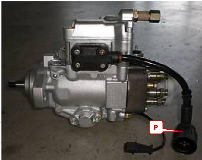
Localise the injection pump and connect the 3061 adapter cable on the 7-pin plug (P).
