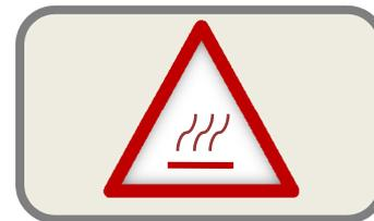
No installation on hot engine parts.
