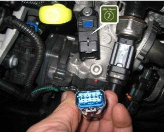
Connect the boost pressure adapter in between both connections.
