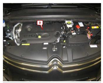
Open the engine hood. Remove the engine cover (D).
