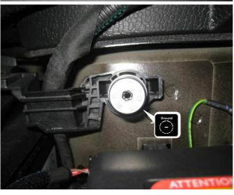
Connect the black cable to the car body mass. Install the adapter cable not in parallel with injection pipelines or ABS-control device connecting leads. Keep to very big distances. Fix the adapter cable with cable binders. Connect the module with the adapter cable. Check all connections again and reassemble the vehicle in reverse order.
