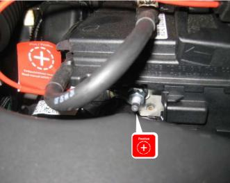
Localise the vehicle battery. Open the flap in front of the battery case. Behind these flap there is the + 12V connection.
