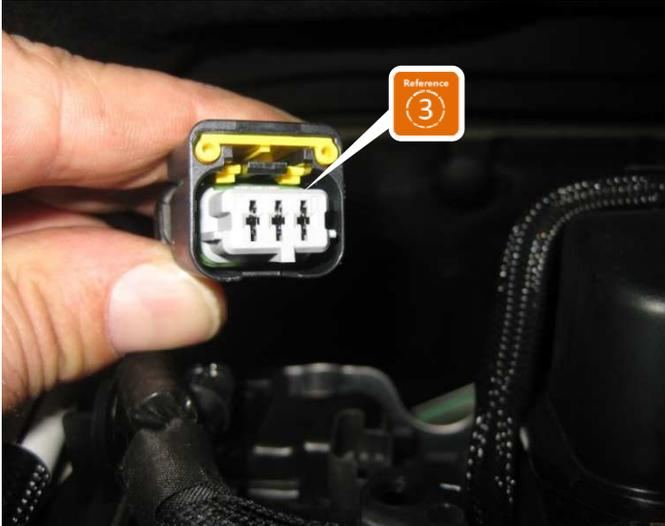
Connect the camshaft signal adapter in between both connections.
