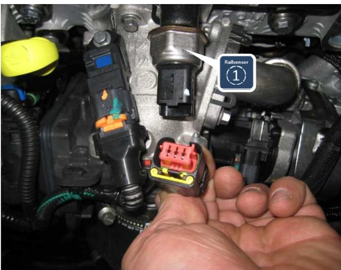
To disconnect the rail pressure plug pull the locking lever. Connect the rail pressure adapter in between both connections.
