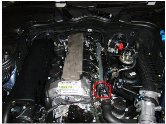
**3.** Pull the 3 pole plug out and connect to the DTUK System to the original connector at the end of the common rail.
