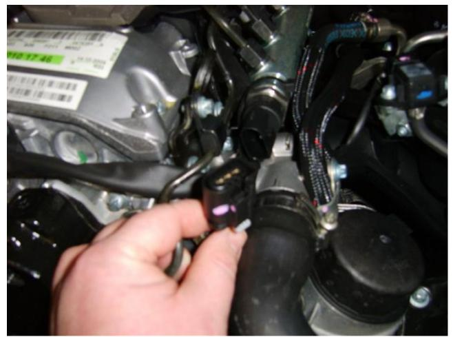
**4.** Now plug the Tuning box into the end of the loom, and replace engine cover and secure the tuning box in a safe place.
