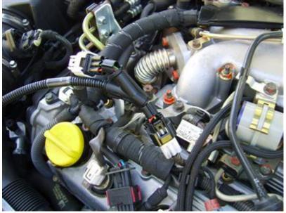
**5.** Connect the tuning box to the wiring loom and replace engine cover making sure no wires are trapped.
