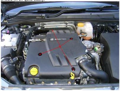
2. Locate the white plastic DN1 connector, just above and to the right of the oil filler cap.
