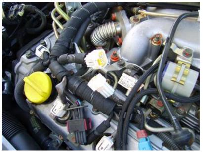
**4.** Connect both ends of wiring loom (supplied with the tuning box) to the male & female connectors in the engine.
