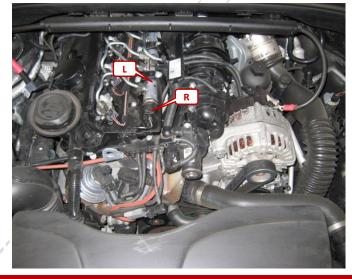
Press the locking device to disconnect the rail pressure plug (R).
