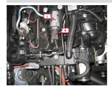
Remove the rail pressure sensor plug ( $\mathbb{R}$ ). Connect the CDI 2 adapter cable with the common rail bar ( $\mathbb{L}$ ). Connect then the original pressure sensor plug with the CDI 2 adapter cable.
