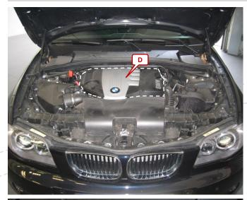
Open the engine hood. Solve the socket head screws (I). Remove the engine cover (D).
