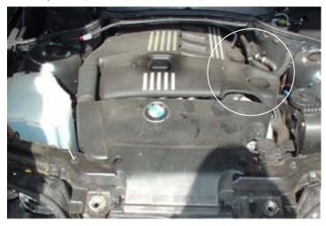
ill.2 installation position VP pump plug
