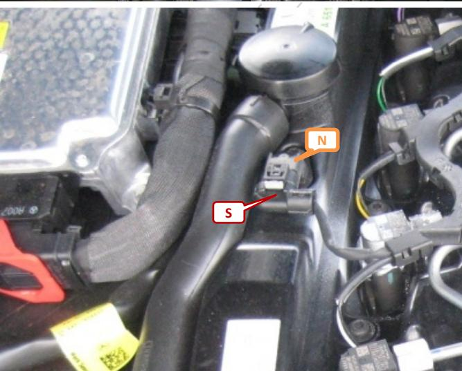
Pull out the locking lever (**S**). Connect the camshaft signal adapter between the both connections.
